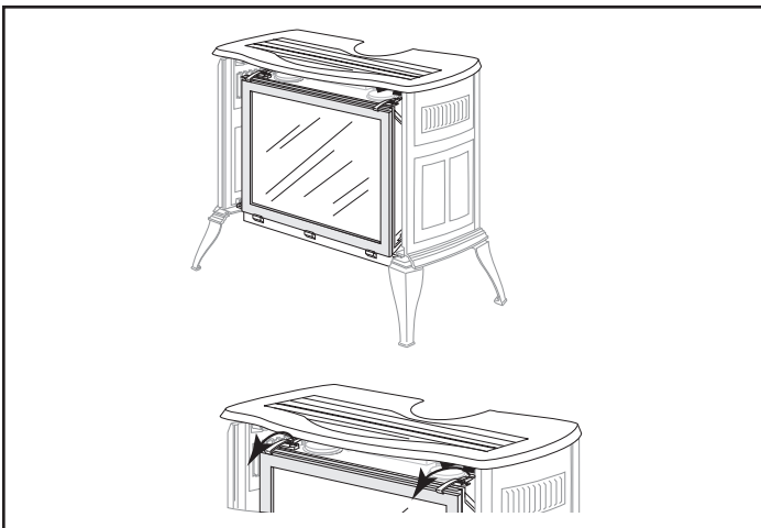
Figure 8.2 - Release the latches to remove the glass frame.
