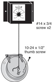
Thumb screw is for manual draft control, to prevent unit from completely shutting down on a low burn. Do not burn hotter than 600 degrees Fahrenheit on furnace top.
