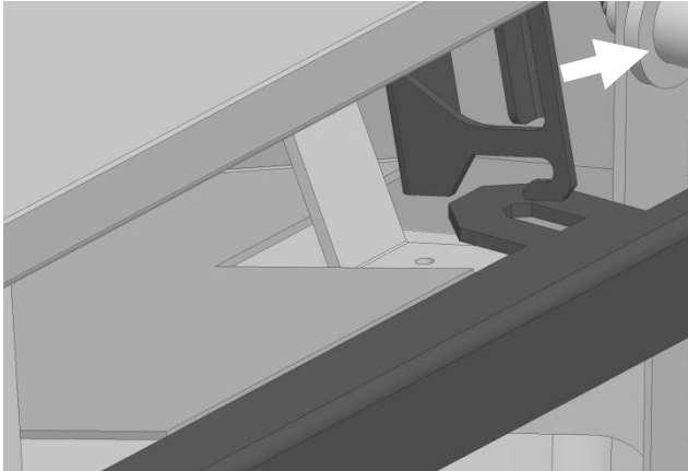
Figure 12 – Glass Frame Upper Mounting Detail
