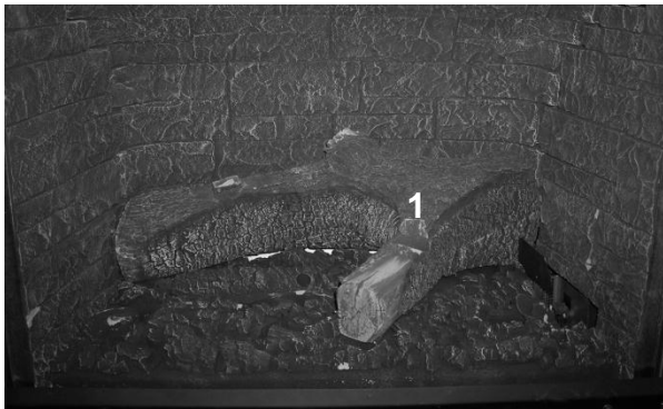
Photo 5 – Log 1 in Position
