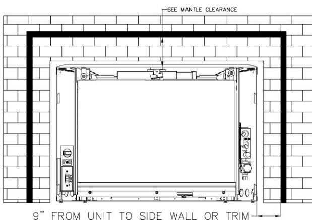
Figure 16 - Minimum Side Trim Clearances
