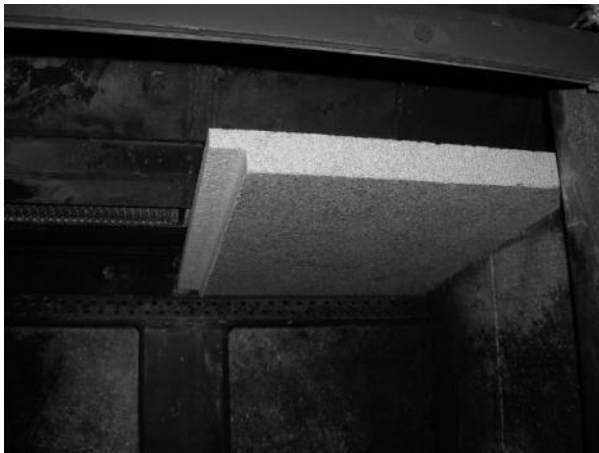
Figure 16 (cont.) - Removing/Replacing the Baffle for Inspection
