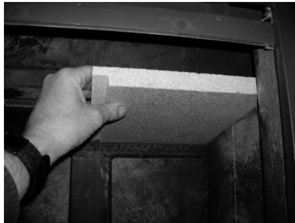
Figure 16 (cont.) - Removing/Replacing the Baffle for Inspection
