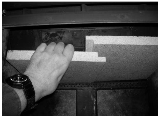
Figure 16 - Removing/Replacing the Baffle for Inspection
