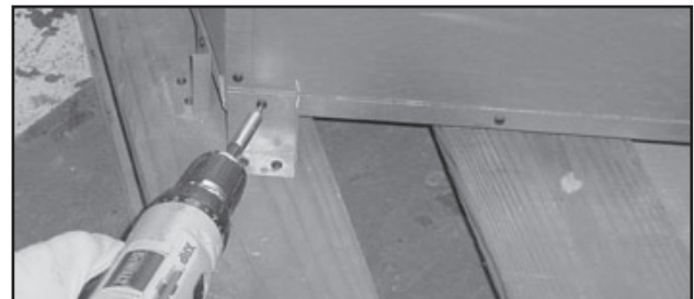
Figure 3.11 Removing Shipping Brackets
