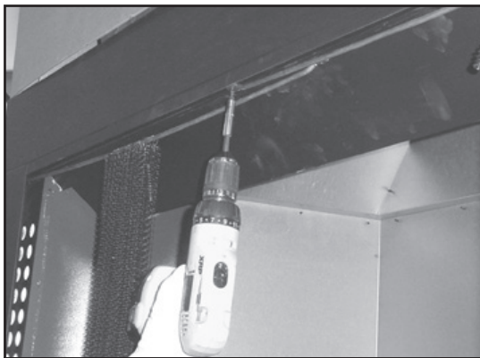
Figure 3.8 Remove Screen Rods
