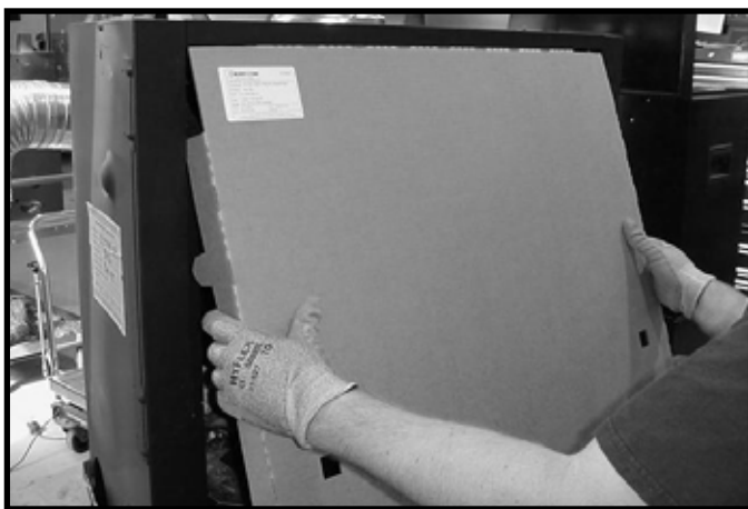
Figure 11.5 Installation of Splatter Guard
