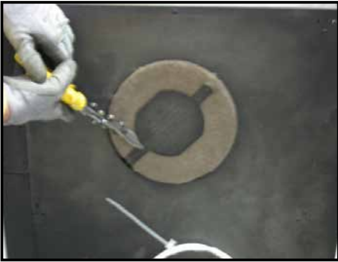
Figure 6.4 Cut the metal retaining band.
