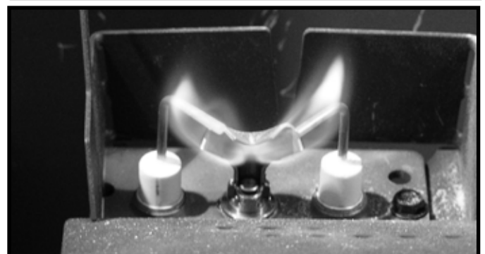
Figure 4.2 IPI Pilot Flame Patterns
