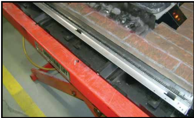
Figure 11.5 Bottom Glass Latch Tabs Installed in Glass Frame
