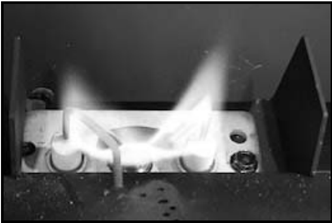
Figure 4.2 IPI Pilot Flame Patterns
