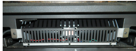
Secure fan with 2 screws removed in Step 1
