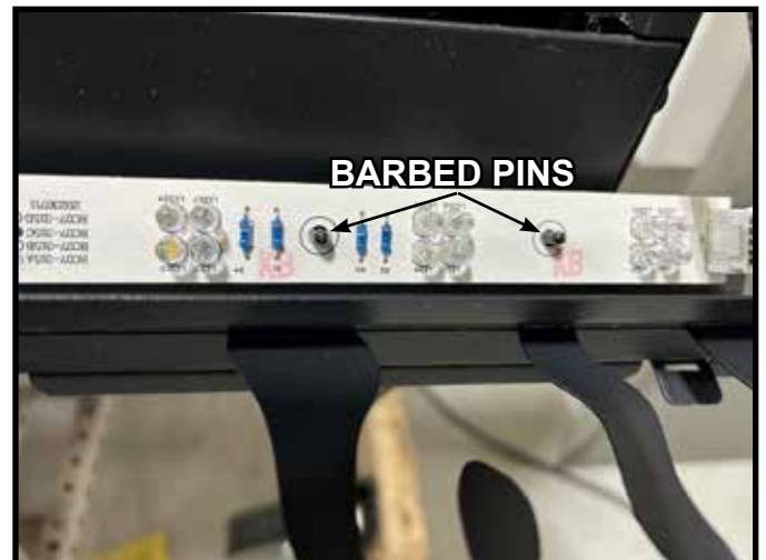
Figure 19 LED Board Removal
