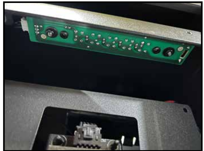
Figure 12 Button Board Bracket Removal
