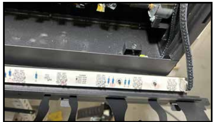
Figure 18 LED Board Attached to Flame Screen Assembly
